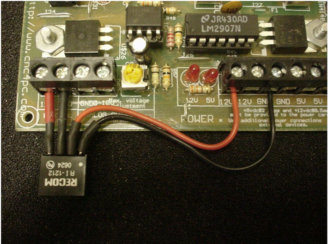
On the right hand side of the board the connections are ground on the power supply to ground, 5 volts to 5 volts, 12 volts to 12 volts.
