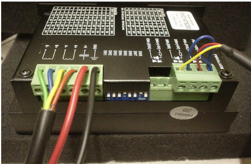
The stepper cable from the motor then goes red to A, yellow to A1, blue to B and green to B1
