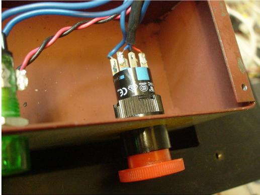
We need to use two terminals that are broken when the switch is pressed. Using the multimeter set to continuity and with one end pin as common find which of the other two pins is broken when the E-stop is pressed. The usual layout is how the other set of terminals are used but double check with a meter. Using the length of twin cable supplied solder a wire to each and thread this cable back through the conduit to exit out the lower panel access.
