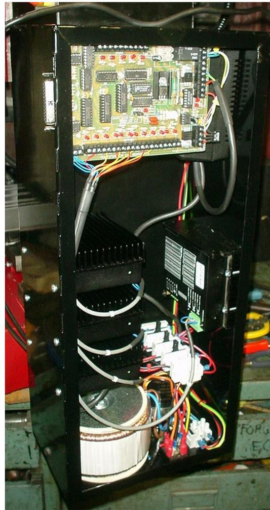
On the output side of the mains fuse holder the brown transformer cable goes to the fused side and the blue cable goes to the opposite end. The centre connection is left empty at this stage for the earth cable when the enclosure is fitted.
