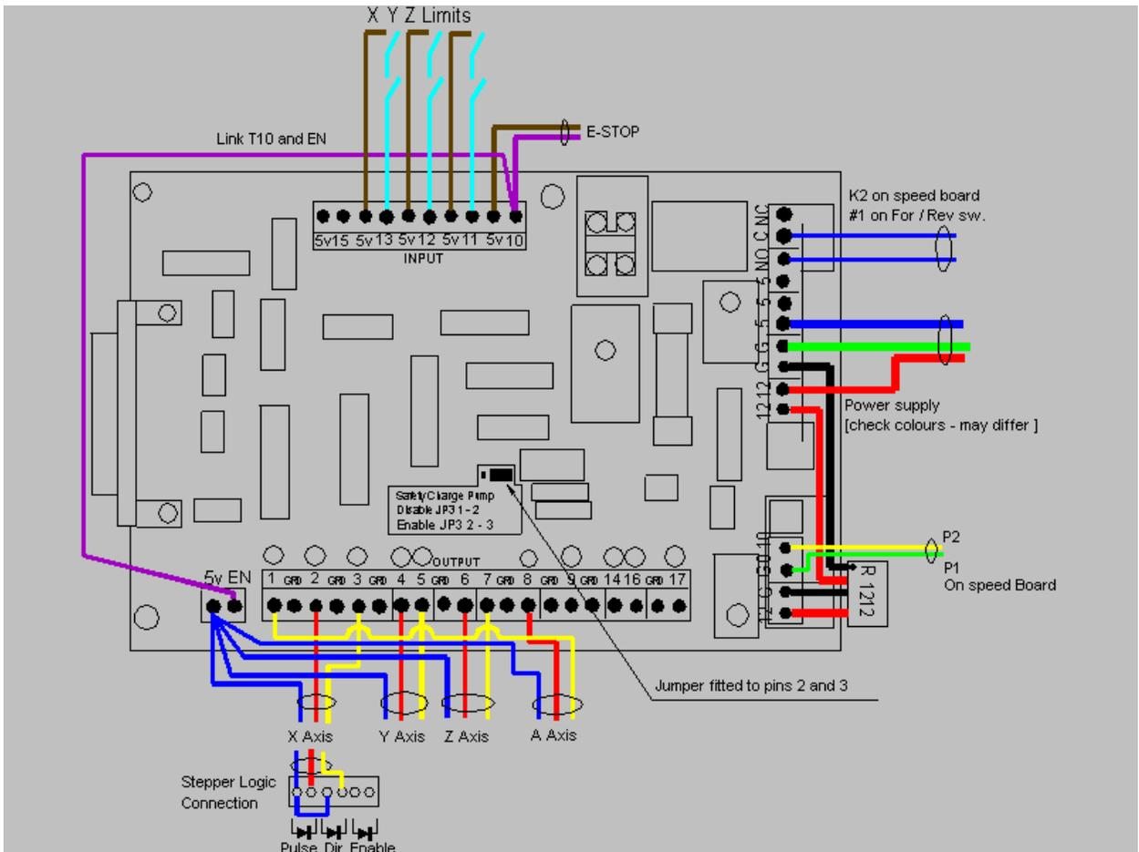
The logic to the stepper drives is carried by three [ or four ] separate light 4 core cabling. Use blue for 5v, red for step and yellow for direction, green is cut back..
