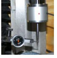
My testing results show excellent repeatability in all axis. Centering of the stylus works well and it eliminates the need to apply offsets in the software.
