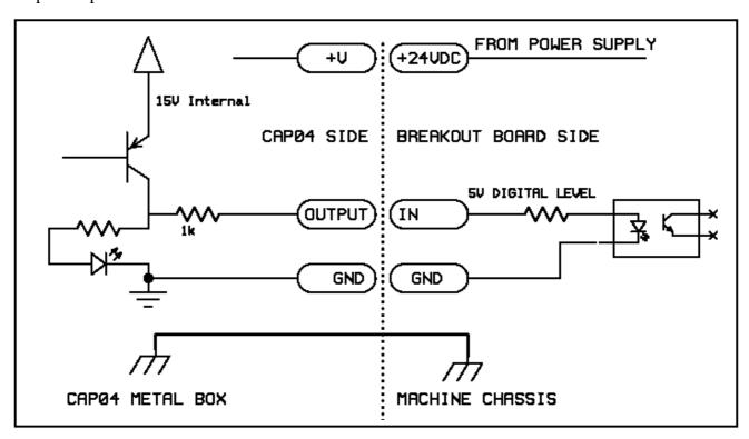
If your BREAKOUT BOARD has 5V digital inputs please use voltage divider <u>resistor</u> as shown below for each inputs.
