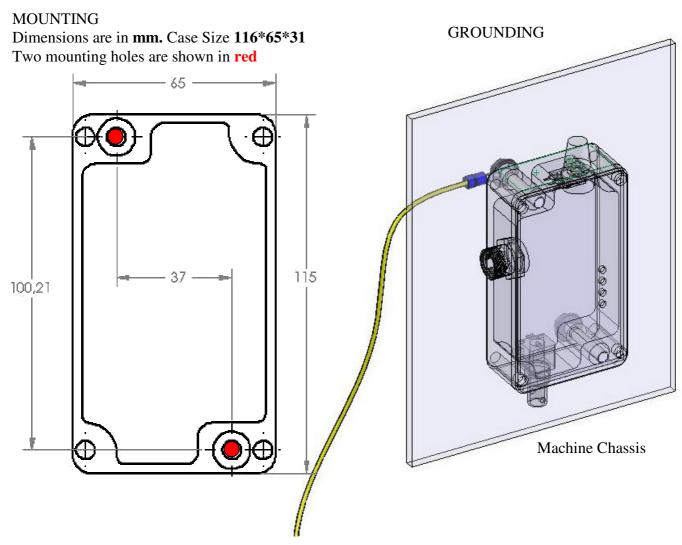
To System & Power Supply Box Use STAR type Ground Connection Use thick wire (10mm²)
