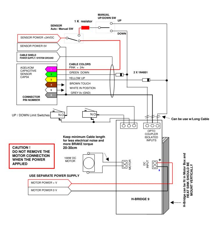
Wiring diagram H-Bridge 9 with BRAKE function
