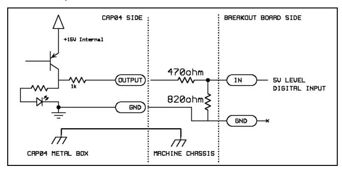
Simplified typical connection of CAP04 sensor is shown below. We advise that using H-Bridge for driving the motor is cost effective. Agelkom H-Bridge-9 Board now available.
