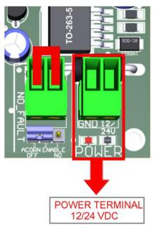
Regulated 12 or +24VDC@200mA is required to power this board.
