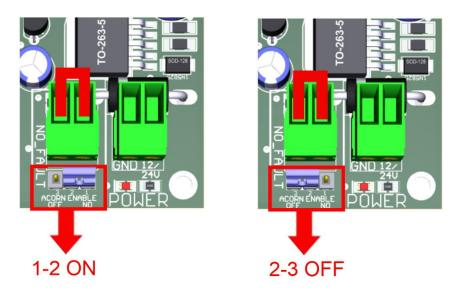
The board can be activated by the axis enable or the NO\_FAULT signal, or a combination of both signals. It could also be hardwired to be permanently active if both inputs are jumped.
