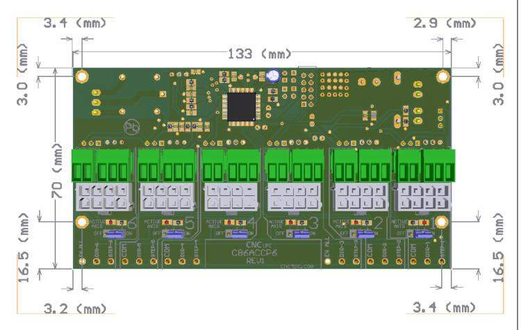
All dimensions are in Millimeters Fixing holes (3 mm)
