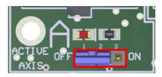
Note: Set the jumper to ON for connected axis and off if no drivers are connected.
